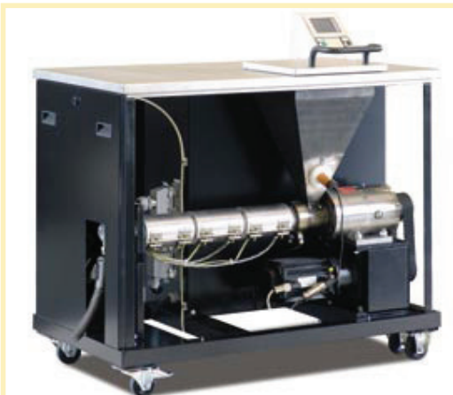
Supply screw including three individual heating zone controls for optimal processing. Filling quantity surveillance via capacitive sensor. Water cooled infeed station. Unlikely to wear out quickly because of crew and housing made of hardened nitrated steel.
